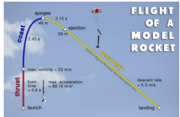
Figure 2 – Flight Path of a Model Rocket
