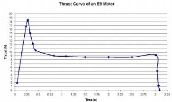
Figure 1 – Thrust curve for E9 motor
