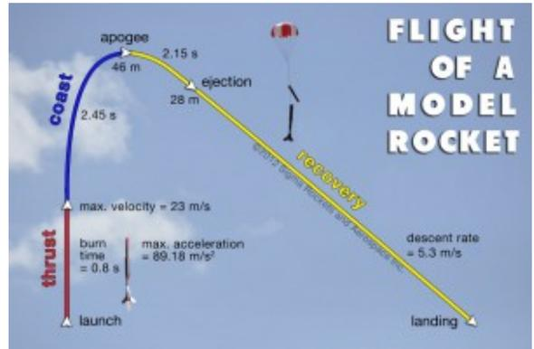
Figure 1 - Flight Path of a Model Rocket
