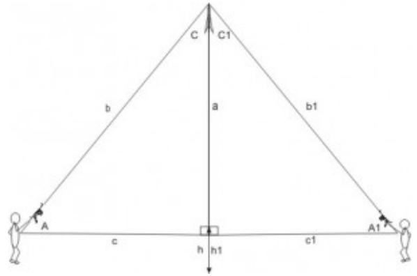
Figure 3 - Using two measurements to determine apogee
