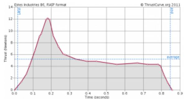
Figure 1 – Thrust Curve of an Estes B6 motor
